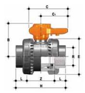
**VXENC**Easyfit 2-way ball valve with female ends, NPT thread
