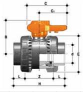
**VXEIC**Easyfit 2-way ball valve with female ends for solvent welding, metric series
