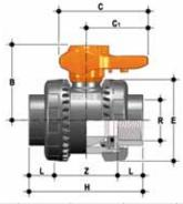
**VXEFC**Easyfit 2-way ball valve with BSP threaded female ends
