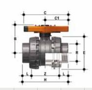
**VXENC**Easyfit 2-way ball valve with female ends, NPT thread
